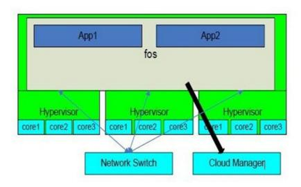
Figure 1. Hypervisor and Network Switch performs the scheduling where FOS communicates with the Cloud Manager to send scheduling command
