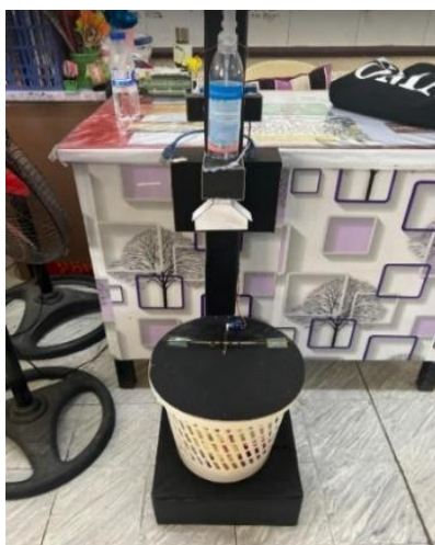
Figure 1. Actual Product of Automated Plastic Trash Bin with Alcohol Dispenser Using PIR Motion Sensor and Arduino Uno
