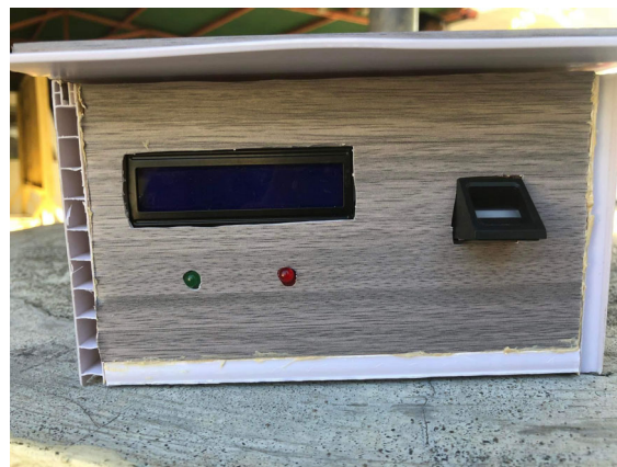
Figure 1. Actual Product of Attendance Management System with a Fingerprint Sensor using Arduino Uno
