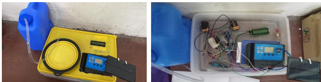
Figure 1. Actual Product of Solar-powered automatic plant watering system with a sensor using Arduino Uno
