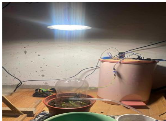
Figure 1. Actual Product of an LED light greenhouse with an automatic water dispenser using Arduino Uno for indoor plants
