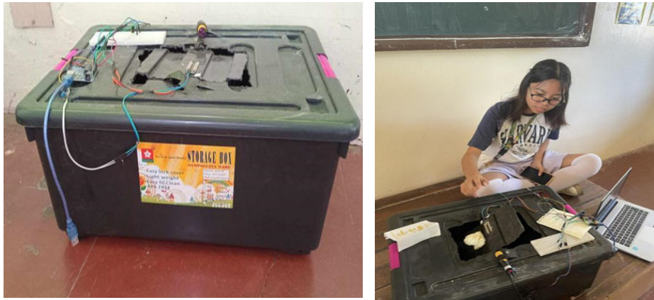
Figure 1. Actual Product of Automated waste segregation system using Arduino Uno R3
