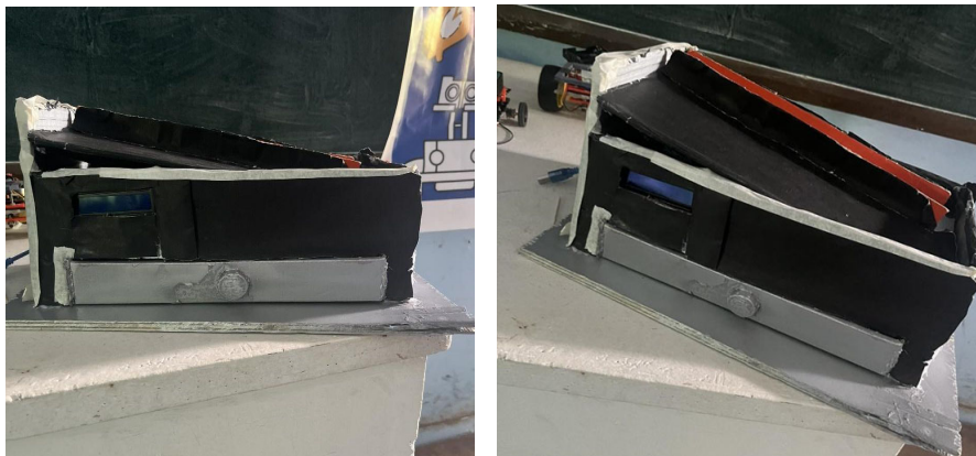
Figure 1. Actual Product of Arduino-Uno-Based automated coin-counting machine
