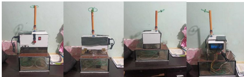
Figure 1. Actual Product of Solar-Powered Pesticide Sprayer using WeMos D1 Arduino-Based Board with Internet of Things Integration
