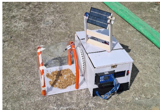
Figure 1. Automated Rice Grain Dryer with Sun Tracking Solar Panel using Arduino Uno
