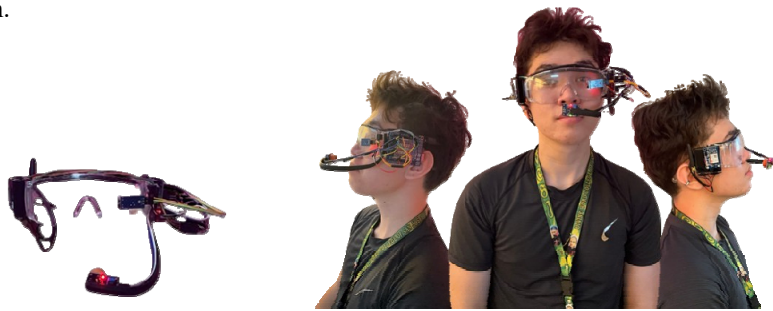
Figure 1. Actual Product of Drowsiness and Alcohol Detection System using Arduino Uno
