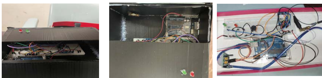
Figure 13. Actual Product Theft Alarm System Using Arduino Uno's P.I.R Motion and Tilt Ball Switch Sensor
