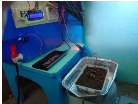
Figure 15. Actual Product of Automated Okra ( Abelmoschus esculentus ) seed germinator using Arduino Uno R3
